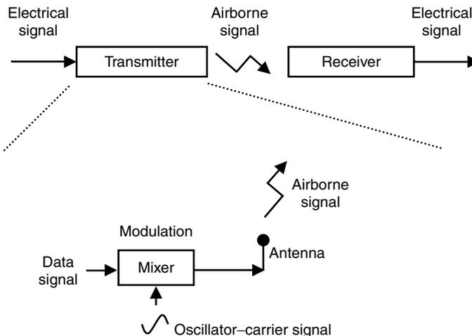
**FIGURE 12.5** Principles of telemetry. (Modified from Weisman, C. J., *The Essential Guide to RF and Wireless*, Prentice Hall, Upper Saddle River, NJ, 2002.)
