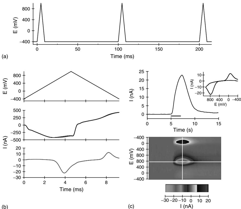
**FIGURE 12.2** (See color insert following page 272.) Fast-scan cyclic voltammetry at a carbon-fiber microelectrode. (a) application of the triangle wave form at 100 ms intervals; (b) current monitored at a CFM during a single voltage scan; (c) voltammetric recording of electrically evoked dopamine release in the striatum of a urethane-anesthetized rat.
