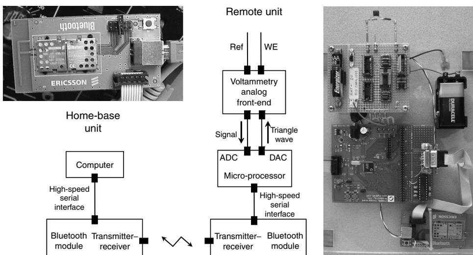
**FIGURE 12.7** Prototype RAT. This large prototype was used to establish proof of principle for the wireless transmission of FSCV at a CFM using RAT. Abbreviations: Ref (reference electrode); WE (working electrode or CFM).
