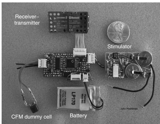
**FIGURE 12.8** Miniature RAT. This small RAT device was used for monitoring electrically evoked dopamine in a freely moving rat.
