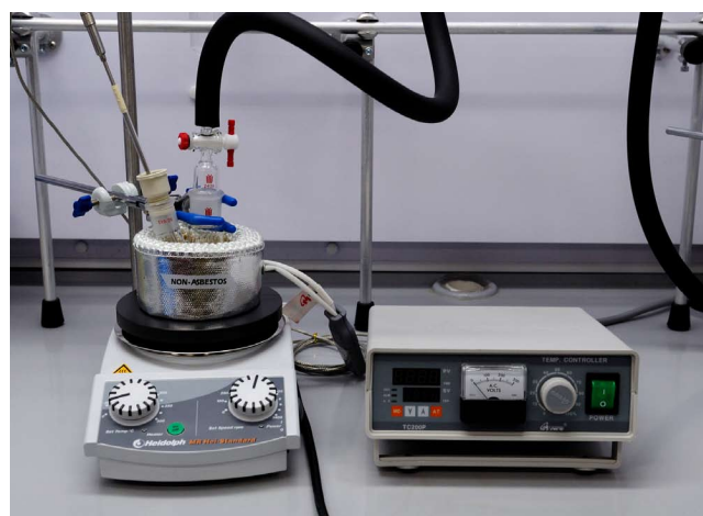
Figure 2 | Photograph of the experimental setup for the preparation of the \text{NaGdF}_4 nanocrystals. Please note that the vacuum/inert gas adapter is not connected to the flask until the reaction mixture is to undergo degassing (see Steps 6, 19 and 32); this process facilitates the removal of the water and methanol added to the reaction mixture as solvents of the reagents. The setup should be placed in a fume hood.
