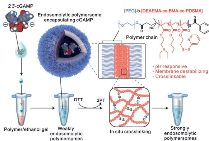
**Figure 3.** (a) Scheme showing STING nanoparticle fabrication and structural details. Adapted with permission from Ref. [14]. Copyright 2019, Nature Publishing Group.
