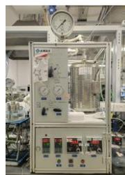
High-pressure Microwave reactor flow reactor
