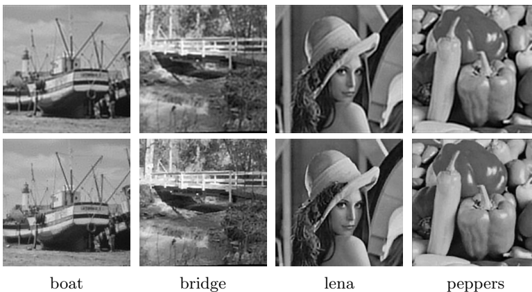
Figure 5: Comparison of deblurred results of sample images blurred by Gaussian blurring kernel ( \sigma=2 ) in the presence of Gaussian white noise with \text{std}=1 . Images shown in the first row and the second row are results using the model from [2] and using our model respectively.
