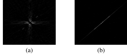
Figure 4. (a) is the cepstrum \mathcal{C}(I) of the blurred image I in Fig. 2 (d) with ramp motion; (b) is the cepstrum \mathcal{C}(I') of the blurred image gradients I' in Fig. 2 (d) with ramp motion.
