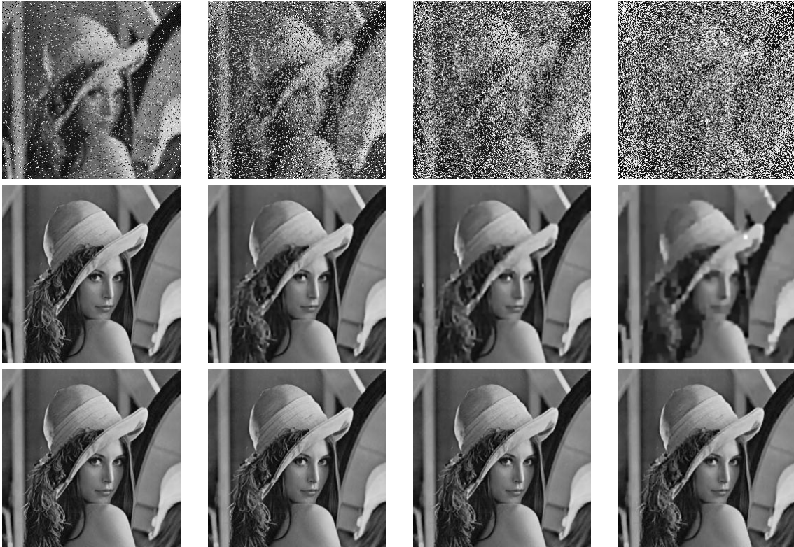
FIG. 3.9. The top row (from left to right) shows the images to be restored, which are blurred by out-of-focus kernel of radius 3 pixels and corrupted consecutively by 10%, 30%, 50%, 70% salt-and-pepper noise. The middle row shows the restored images by the full variational algorithm; the corresponding PSNR values are 36.09, 29.84, 27.58, 24.13 respectively. The bottom row shows the restorations by the two-phase algorithm; the corresponding PSNR values are 42.51, 38.60, 35.08, 31.65 respectively.
