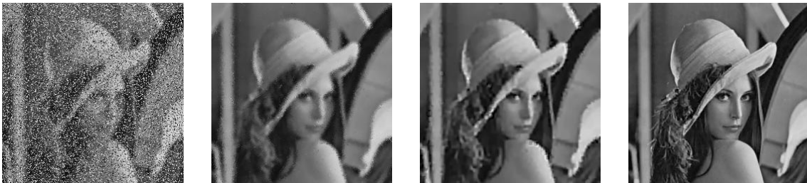
FIG. 3.11. From left to right shows the corrupted image with the out-of-focus kernel of radius 3 pixels and 40% random-valued impulse noise, the intermediate output from median filtering, the restoration by using \ell_2 -norm based data fidelity term in (3.5) and the restoration by using \ell_1 -norm based data fidelity term in (3.5).
