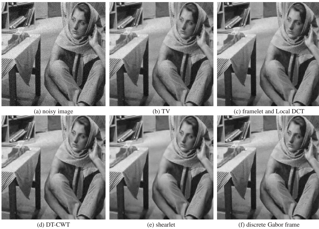
Fig. 8 Visual illustration of image denoising. (a) noisy image with noise level \sigma = 20 ; (b)-(f) denoised results by five different methods.
