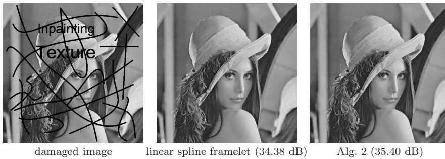
Fig. 7 Visual comparison of in-painted results for the image "Lena512". Some image pixels of the true image are damaged by the scratches and texts.
