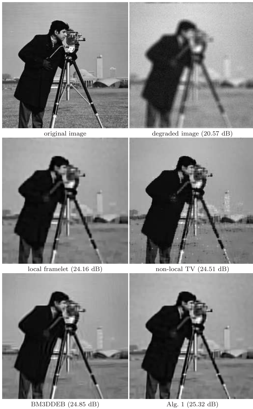
Fig. 3 Visual comparison of de-blurred results for the image "cameraman256". The true image is degraded by the 9 \times 9 box kernel and the Gaussian noise with standard deviation \sigma = 5 .
