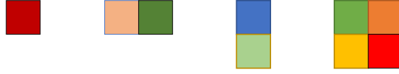
FIGURE 3. Phantom shapes for simulated data, each cubic container is of size 5mm \times 5mm \times 5mm ( 1 \times 1 \times 1 voxel).
