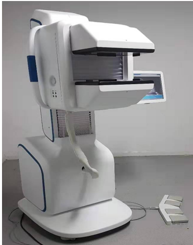
FIGURE 1. A prototype time-resolved diffuse optical tomography system designed for optical imaging of human breast [25]
