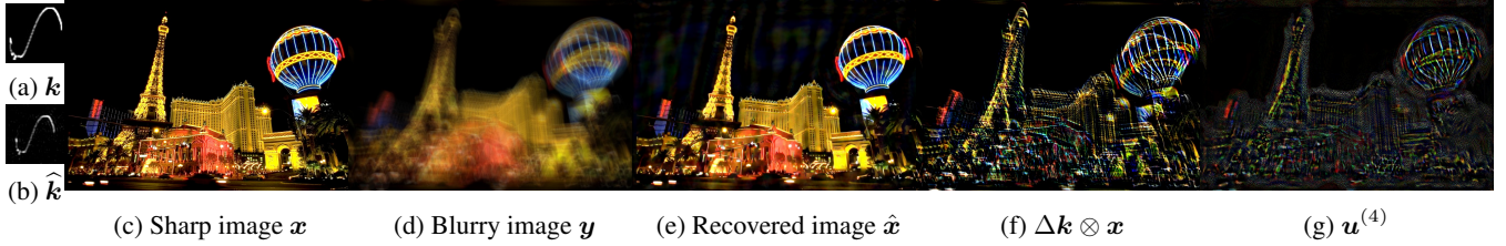
Figure 2: Visualization of the output of DP-Unet u in Stage S_4 of one example, in comparison with the ground truth correction term \Delta k \otimes x . (a) Ground truth kernel. (b) Noisy kernel. (c) Sharp image x . (d) Blurry image y . (e) Recovered image \hat{x} . (f) Ground truth correction term. \Delta k \otimes x . (g) Predicted correction term u^{(4)} .
