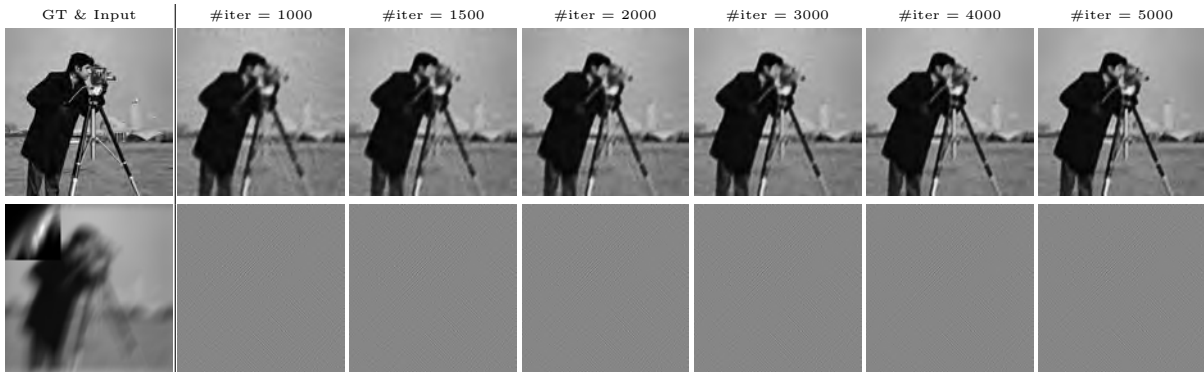
Fig. 1 Illustration of the prediction error in the approximate null space at different iterations of DIP. The top row shows the output images over different iterations. The bottom row shows the the errors in the approximate null space. It can be seen that there are some artifacts around the cameraman' head and the camera tripod, along the learning process.
