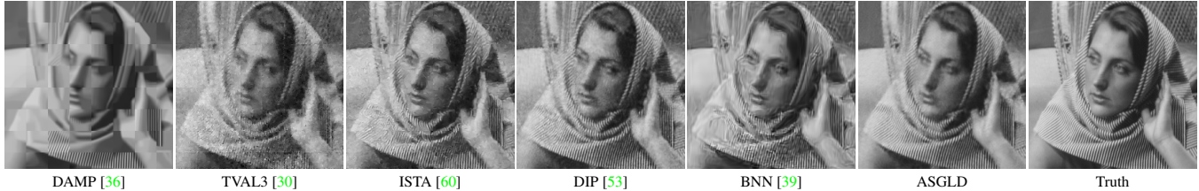
Figure 3. Results of CS image reconstruction using noisy input with ratio 25% for “Barbara”.
