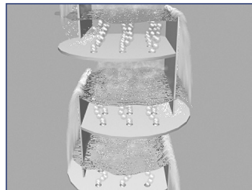
Screen capture of a video demonstrating vapour-liquid mixing: sieve tray in a distillation column
