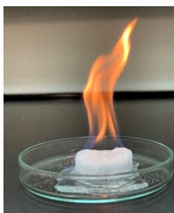
Burning SNG pellet synthesized at Linga Lab
