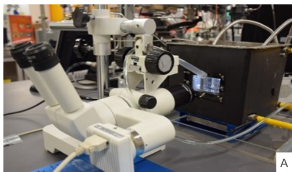
(A) Morphology setup; (B) Needle-shape semiclathrate hydrates observed by microscope
