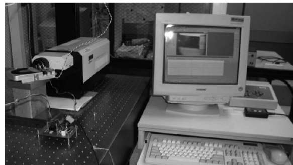
Fig. 2. Experimental setup. HDD (left), LDV-laser unit (left), VCM-driver (center-left), LDV-control-unit (PC right).
