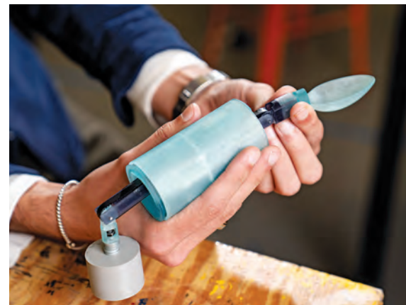
LEFT Raleigh Dewan and Mason Morland discuss how the mechanics of StediSpoon enable stability for those who suffer from tremors; RIGHT a prototype of the StediSpoon.
