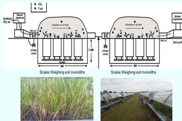
Figure 1. Experimental setup diagram (Fay et al., 2009) and pictures from Lysimeter CO<sub>2</sub> gradient (LYCOG) facility in USDA-ARS at Temple, TX
