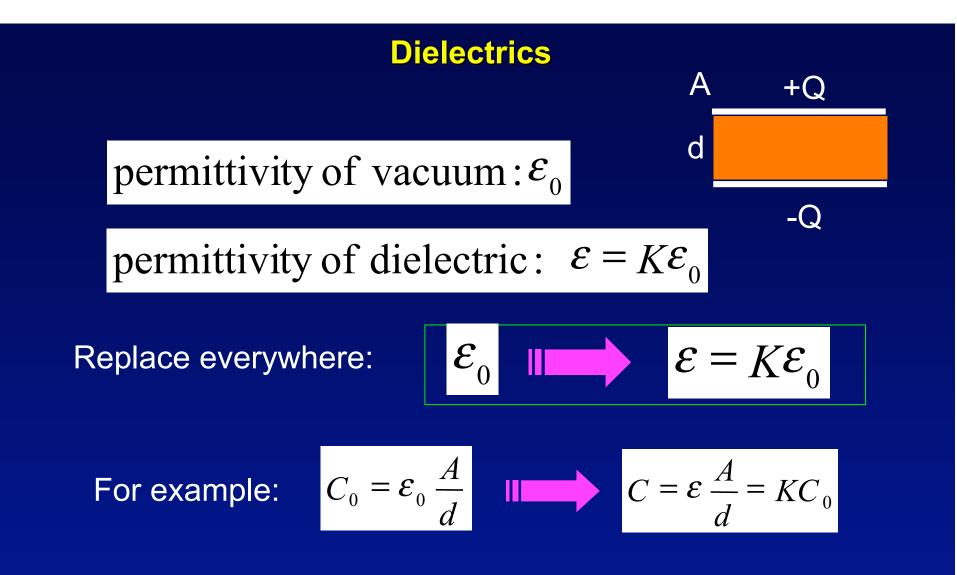
For constant Q, electric field  $E_0 = \sigma/\epsilon_0$ . With dielectrics:  $E = \sigma/\epsilon$ = $E_0/K$ . Then V=Ed=V<sub>0</sub>/K. Then U=1/2 CQ=K U<sub>0</sub>.
