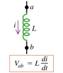
(b) Inductor with current *i* flowing from *a* to *b*:
