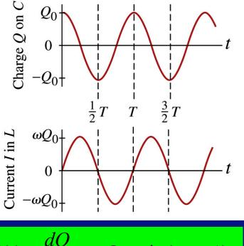
$I(t) = \frac{dQ}{dt} = -Q_0 \omega \sin(\omega t + \phi)$
