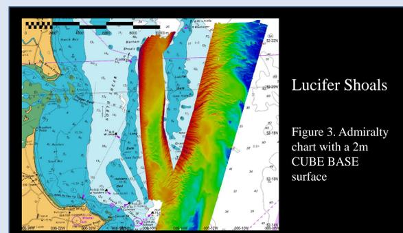
Figure 3. Admiralty chart with a 2m CUBE BASE surface
