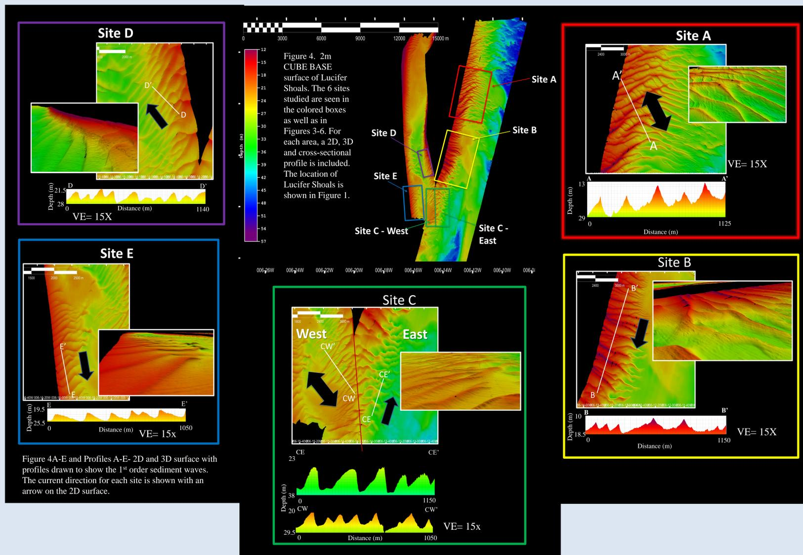
Figure 4. 2m CUBE BASE surface of Lucifer Shoals. The 6 sites studied are seen in the colored boxes as well as in Figures 3-6. For each area, a 2D, 3D and cross-sectional profile is included. The location of Lucifer Shoals is shown in Figure 1.
