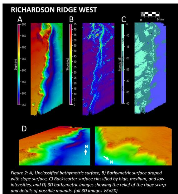
Figure 2: A) Unclassified bathymetric surface, B) Bathymetric surface draped with slope surface, C) Backscatter surface classified by high, medium, and low intensities, and D) 3D bathymetric images showing the relief of the ridge scarp and details of possible mounds. (all 3D images VE=2X)
