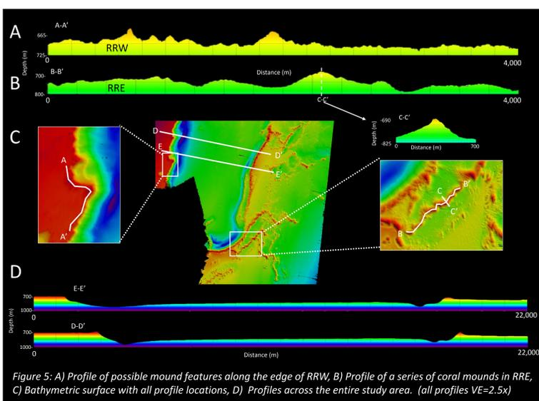
Figure 5: A) Profile of possible mound features along the edge of RRW, B) Profile of a series of coral mounds in RRE, C) Bathymetric surface with all profile locations, D) Profiles across the entire study area. (all profiles VE=2.5x)
