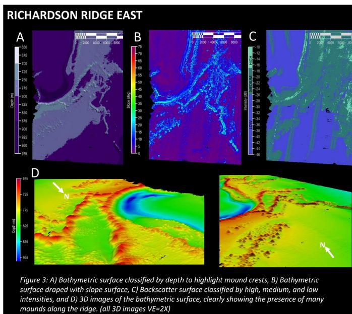
Figure 3: A) Bathymetric surface classified by depth to highlight mound crests, B) Bathymetric surface draped with slope surface, C) Backscatter surface classified by high, medium, and low intensities, and D) 3D images of the bathymetric surface, clearly showing the presence of many mounds along the ridge. (all 3D images VE=2X)
