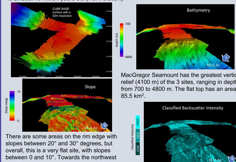
There are some areas on the rim edge with slopes between 20° and 30° degrees, but overall, this is a very flat site, with slopes between 0 and 10°. Towards the northwest area of the seamount, there is a cliff face that has a steep drop from 1500 to 2500 m with slope approaching 70° in some parts.
