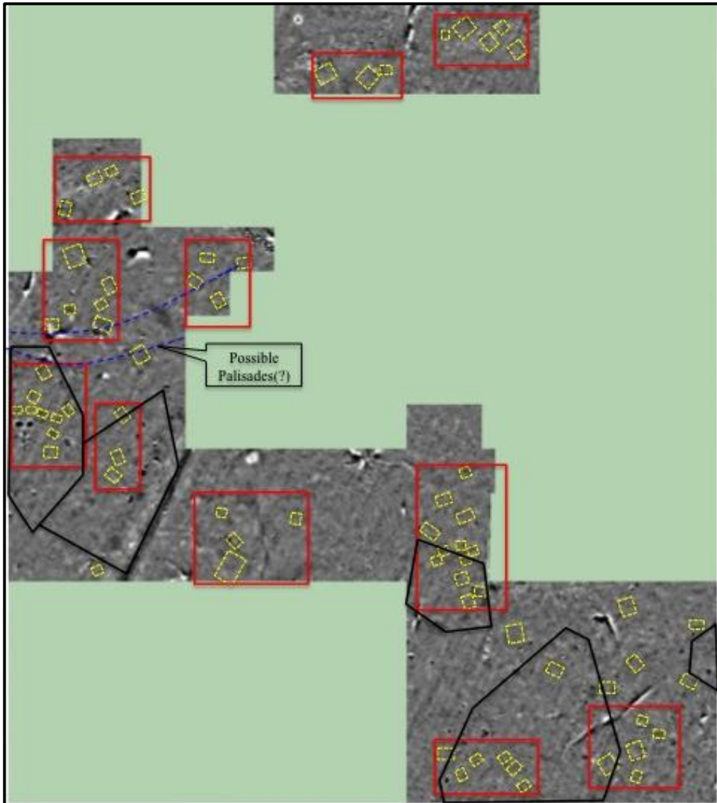
Figure 10. Magnetometry data ( \pm 6 nT) with 70 interpreted structures mostly in clustered groups (red) as well as possible palisades. Recorded artifact scatters (black) tend to correlate with clusters of structures.
