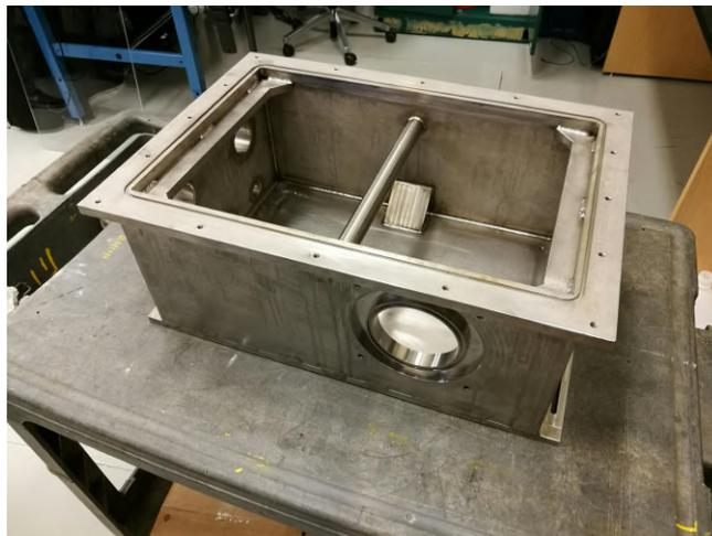
FIGURE 3.13: Photograph of the manufactured pre-chamber. Tests are currently being performed in order to ensure it presents no leaks before moving it onto the optical table.
