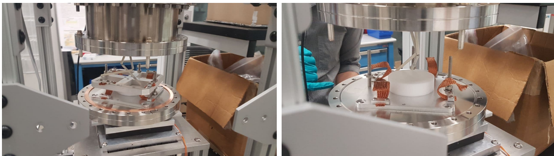
Figure 4.26: Pictures of installing a PTFE sample into the outgassing setup.
