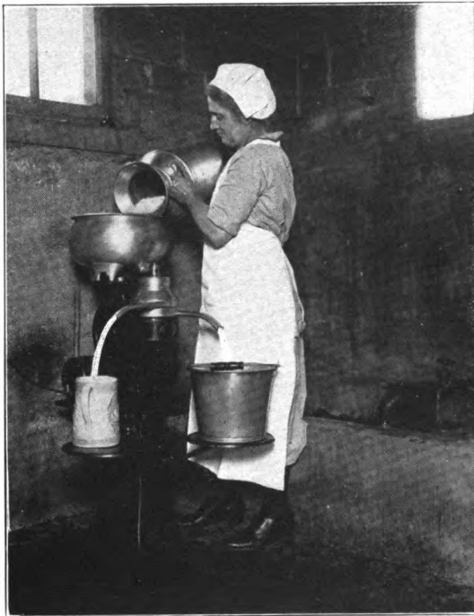
Figure 19. The cream separator, to obtain its most successful operation, must be driven at a uniform rate of speed. The electric motor, with its constant speed, replaces other types of power for driving the separator when electricity is available. One of the commonest uses of an electric motor on the farm is to drive the cream separator, as it is doing on this Tippecanoe County farm. Two thousand pounds of milk are separated by 1 K. W. H. of electrical energy costing 13c, as shown by the average of a number of tests.
