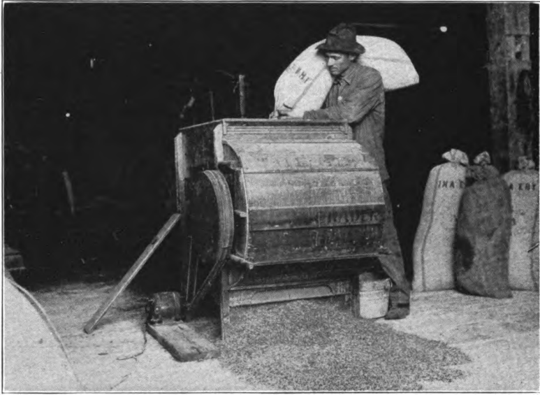
Figure 16. The use of a quarter H. P. motor frequently saves the labor of an extra man on the farm. An Elkhart County farmer has mounted a motor of this size on a short piece of plank to assist in transporting and operating it. The motor has replaced a windmill for pumping water and is also used for odd jobs such as is shown in the picture. A motor of this size will operate from 3 to 4 hours with a consumption of 1 K. W. H. of electrical energy costing 13 cents.
