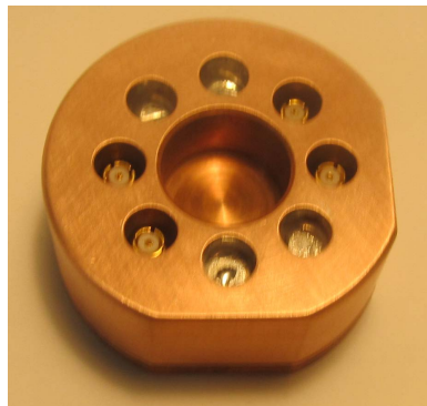
Figure 3.2: Octobox sample holder, closed. The eight holes of the top of the lid can be seen. The connectors on the PCB can be seen in four of the holes. The other four holes are plugged to prevent additional infrared radiation from reaching the sample.
