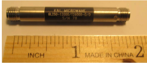
Figure 3.14: K&L low-pass microwave reflection filters. They pass microwaves below a cutoff frequency (the filter shown here is 12 GHz) and are specified to reflect all other incoming frequencies up to 26 GHz.
