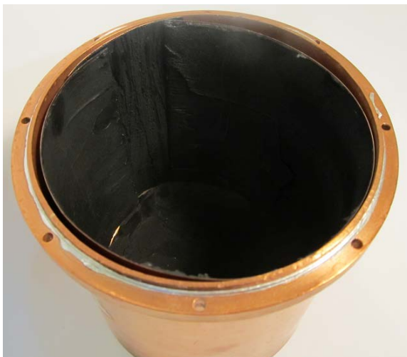
Figure 3.19: Image showing inside of infrared shield can. An infrared absorbent coating was applied to a thin copper sheet and placed on the walls and bottom of the can. The remaining indium seal between the can and the plate of the infrared shield can also be seen here.
