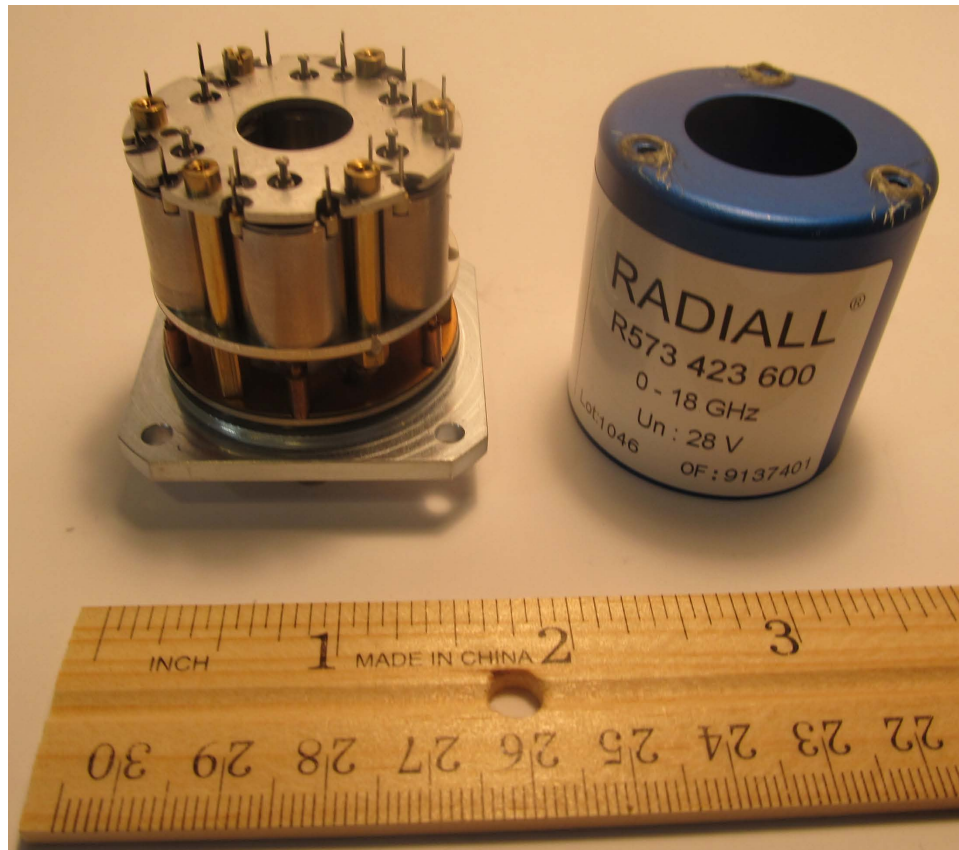
Figure 3.12: Radiall SP6T switch, modified to work at low temperatures inside of a dilution refrigerator. On the left is the switch, with PCB removed and connectors glued in place. On the right is the body of the switch, removed to show the details inside.
