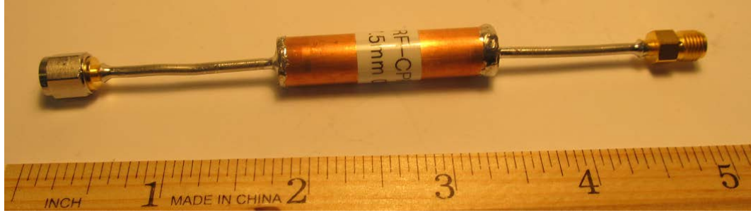
Figure 3.17: Picture of copper powder filter showing typical length for a filter with 2 dB loss at 10 GHz.
