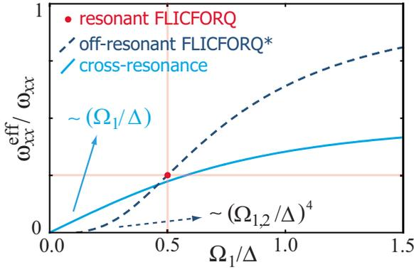
FIG. 2. (Color online) Effective interaction strength generated by cross-resonance driving as a function of drive strength-to-detuning ratio  $\Omega_1/\Delta$  (solid); generalized off-resonant FLICFORQ scheme of Refs. 15 and 17 (dashed); and double-resonant driving of original FLICFORQ (Ref. 14) (red point). Equal drive amplitudes ( $\Omega_1=\Omega_2$ ) on each qubit are assumed for the latter two.
