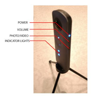
The Theta camera takes 360 photos and videos that can be viewed on computers and with VR goggles. There is a Theta application for mobile devices that allows one to connect to the camera wirelessly. It is possible to view photos on your mobile device and use it as a remote for the camera. Above is the camera with the buttons on the side. Turn on the power, select the photo or video button and wait for the blue indicator lights on the front.
