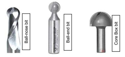
**Ball** – Ball bits are used to give a radius to the inside corners of pocket cuts. When used for 3D projects with low percentage stepovers, the radii help blend each path together, resulting in less finish work. A ball nose bit is a poor choice for profile cuts as the bit will have to go past the bottom of the material the radius of the bit into the spoilboard to get a clean profile.
