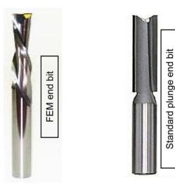
**Standard End** – bits will plunge cut nicely, these bits can be identified by the swallow tail style profile of the end of the bit. This bit is the right choice when cutting profiles. The disadvantage of this style bit is it leaves marks or swirls when pocket cutting.
