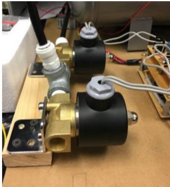
Figure 9: The two solenoid valves (black, cylindrical units w/brass valves); background unit (intake), foreground unit (exhaust)
