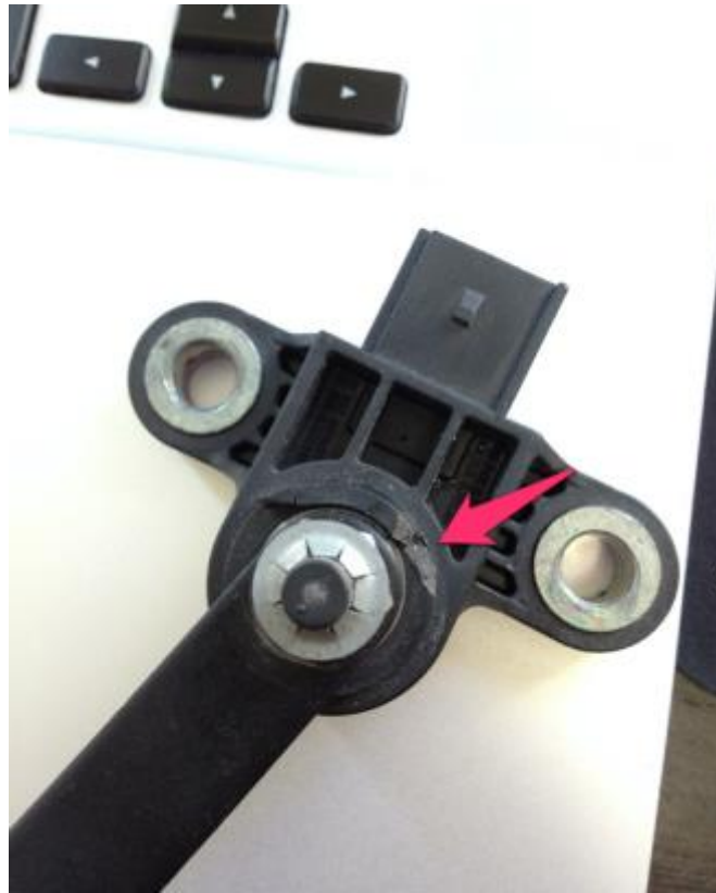
Figure 4: A broken height sensor; arrow points the damaged area.
