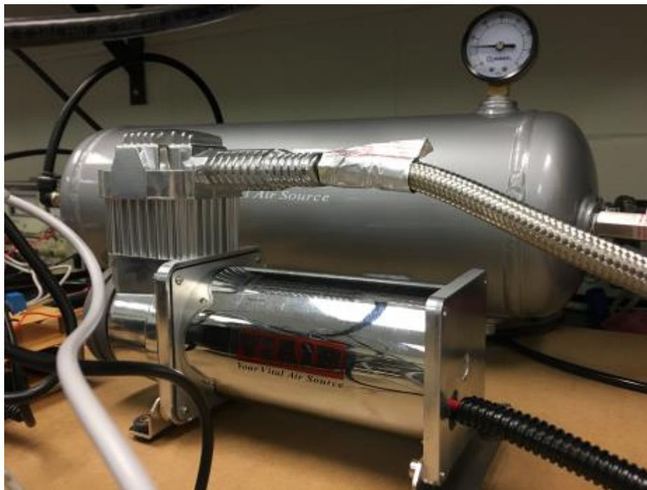
Figure 11: The VIAIR 380C in the foreground, with the 2 gallon air tank in the background
