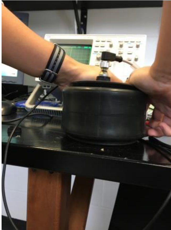
Figure 10: Air House 2, compressed, no internal pressure, w/UK6 rangefinder, w/o air line
