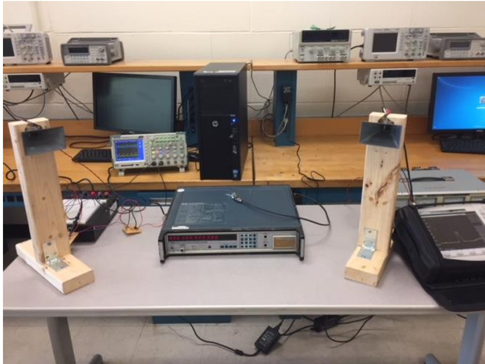
Figure 18. Image of functional radar final system and test setup
