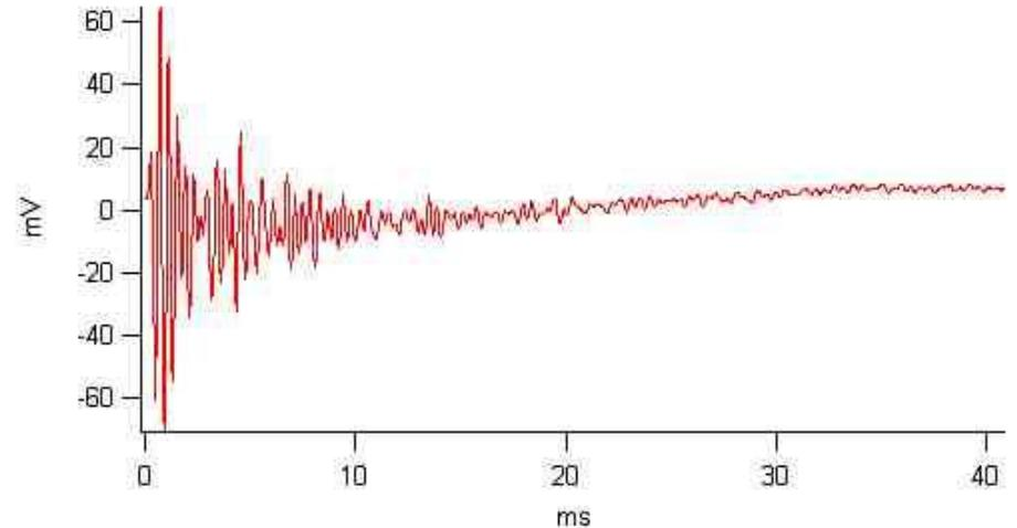
Shown (left): deflection impulse response to a 4V discrete voltage change to z piezo
