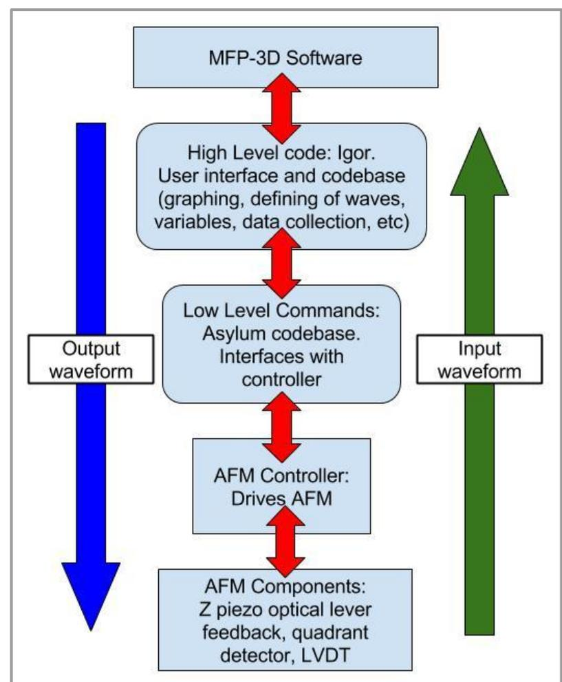
Block diagram for system I/O
