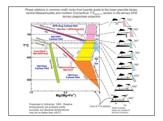
This is a ~6 kbar T-Mg' section through the above series of phase diagrams showing the solid solution gaps between different coexisting phases.
