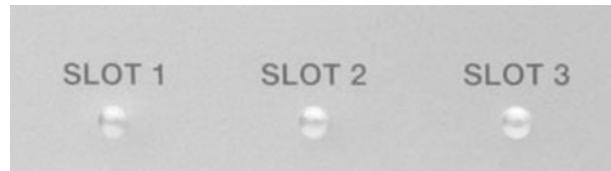
Fig. 17: LEDs for active slots of CCU 1000
