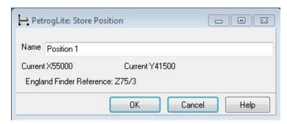
The current position can be stored so that the **SteppingStage** can later be sent back to this position.
