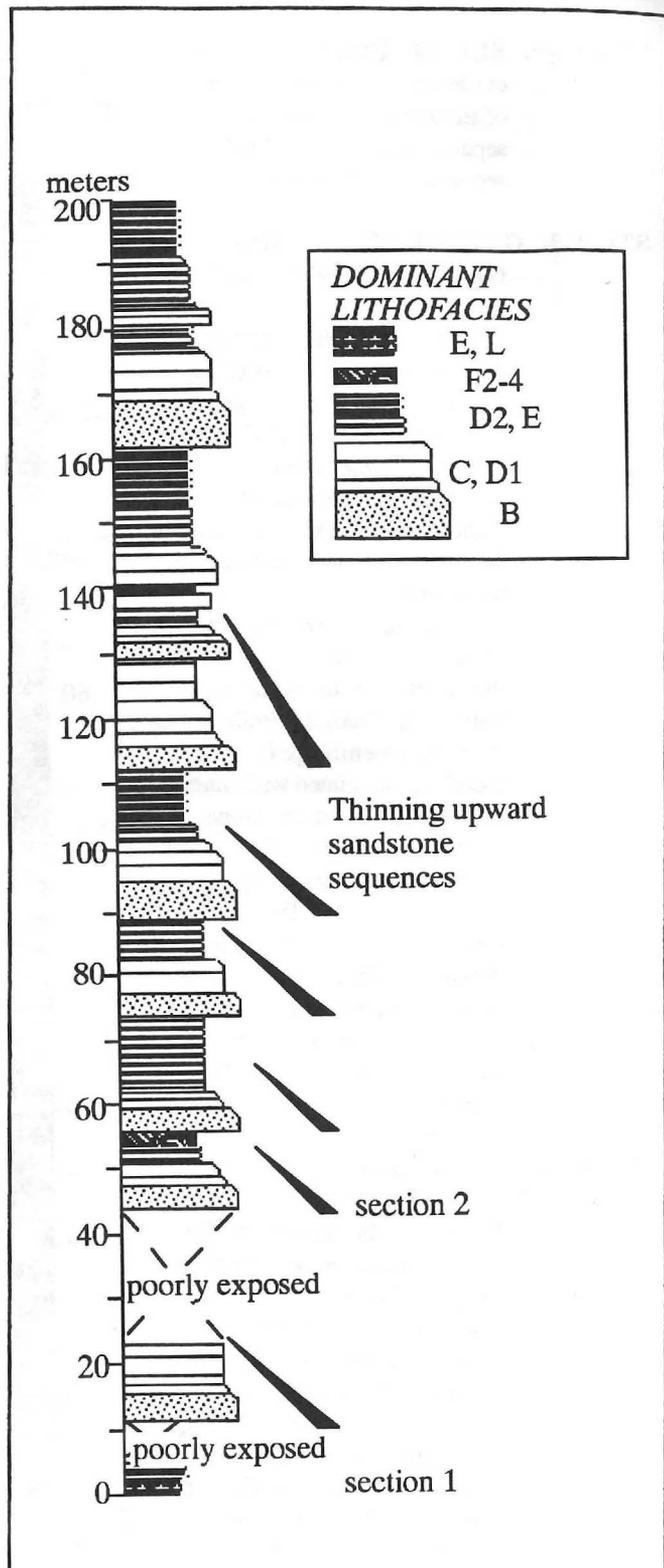
Figure 4. Schematic column of crude thinning-upward sandstone sequences in the Gauntlet Falls section.
