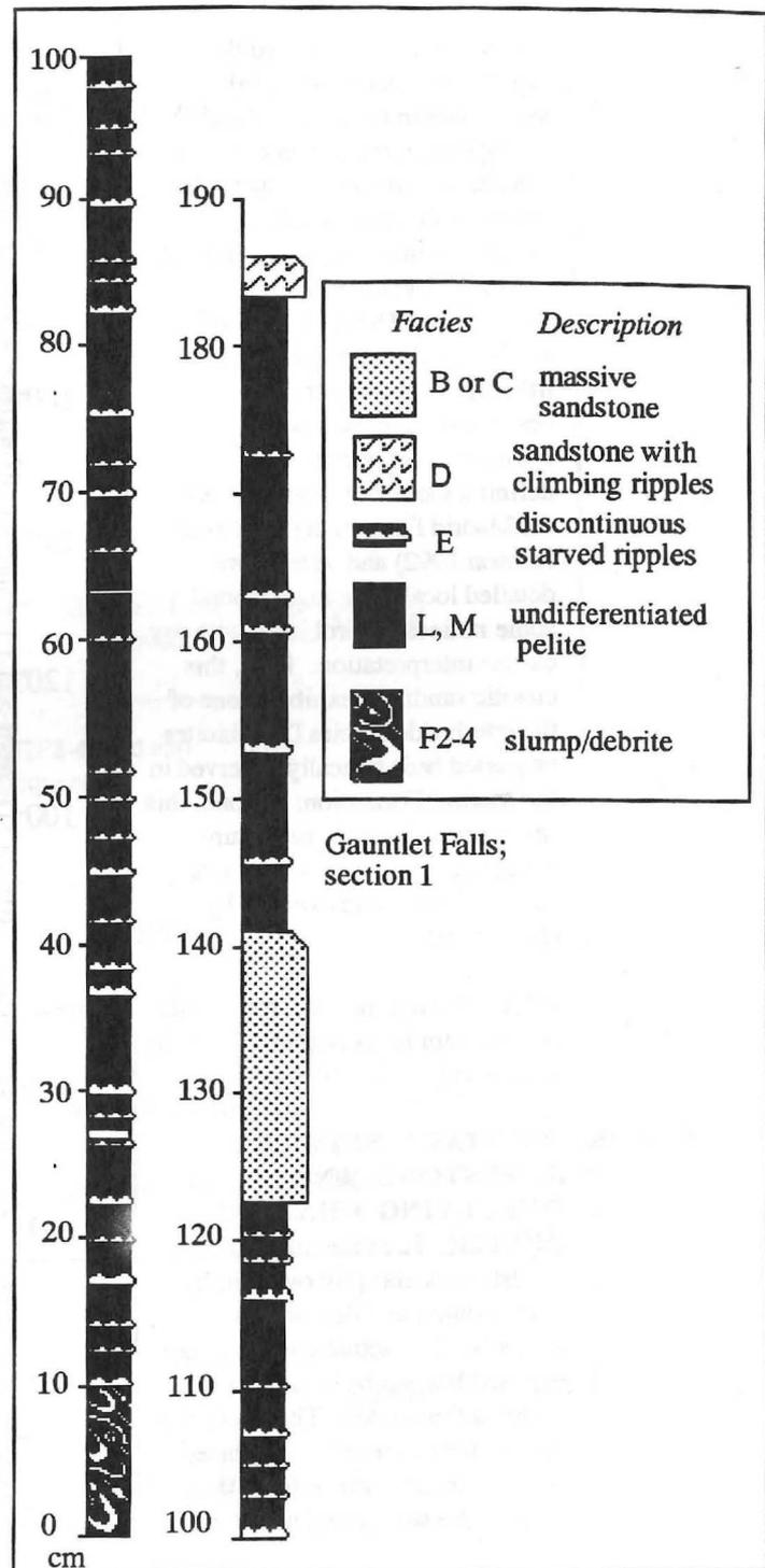
Figure 5. Detail of pelites and thin-bedded sandstones overlying debris flow at Gauntlet Falls.
