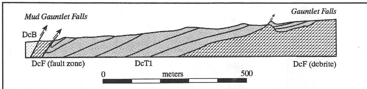
Figure 7. Cross-section of the Carrabassett Formation between Gauntlet and Mud Gauntlet falls (After Hanson 1988). Strata are labeled as follows: DcF (disrupted beds), DcT (thin and thick-bedded sandstone-rich turbidites), and DcB (massive sandstone).
