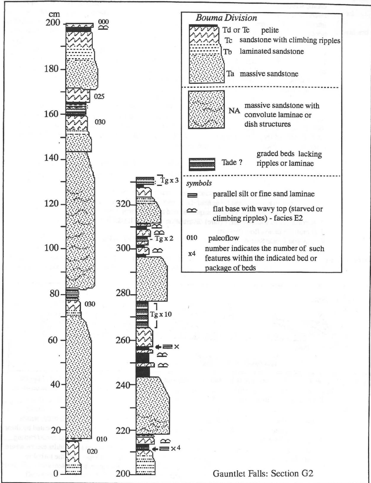
Figure 6. Detailed section of thinning-upward sequence within the Gauntlet Falls Section.
