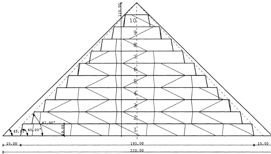
Fig. 15. Arrangement of ramps for the construction of the core of the Red Pyramid.
