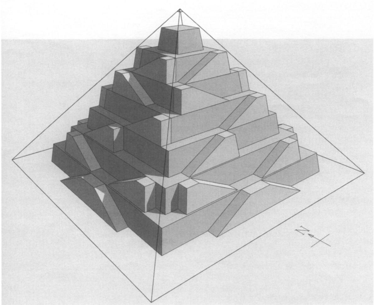
*Fig. 11. Ramps used for construction of the stepped core (perspective drawing).*
