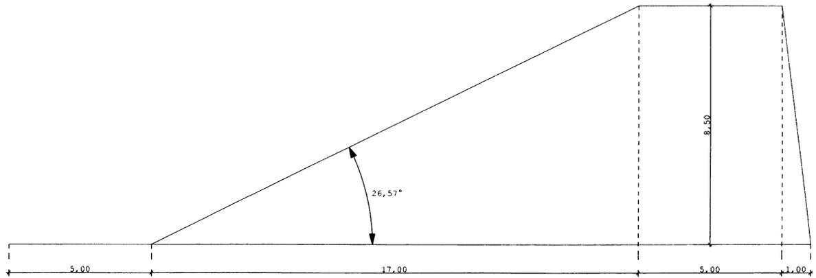
Fig. 8. Suggestion for a transport ramp.
