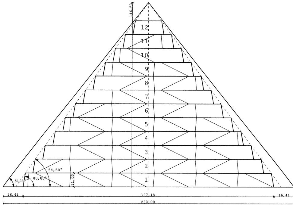
Fig. 16. Arrangement of ramps for the building of the core of the pyramid of Khufu.
