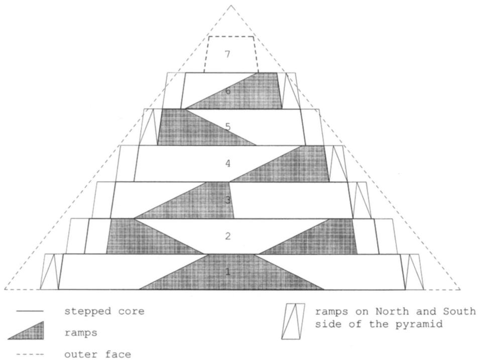
Fig. 9. Arrangement of ramps on the first to sixth core step.
