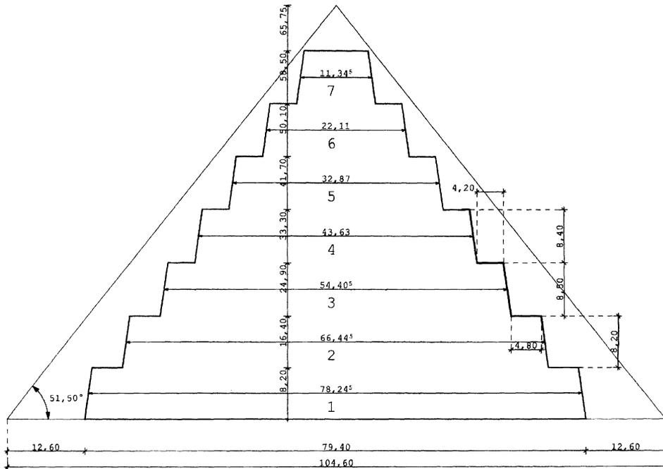
Fig. 7. Stepped core of the pyramid of Menkaure.
