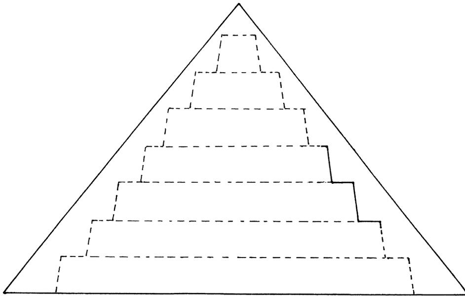
Fig. 6. Cross-section (S-N) of the pyramid of Menkaure with steps archaeologically attested in the breach on the north face (drawn lines) and the other steps of the core reconstructed by analogy (dotted lines).
