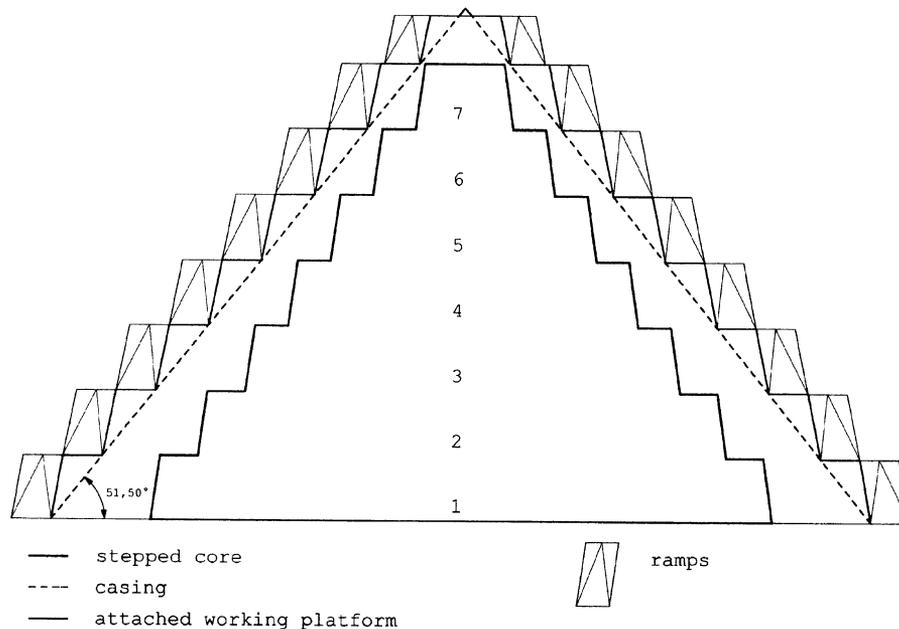
Fig. 13. Working platforms attached to the faces of the pyramid of Menkaure.
