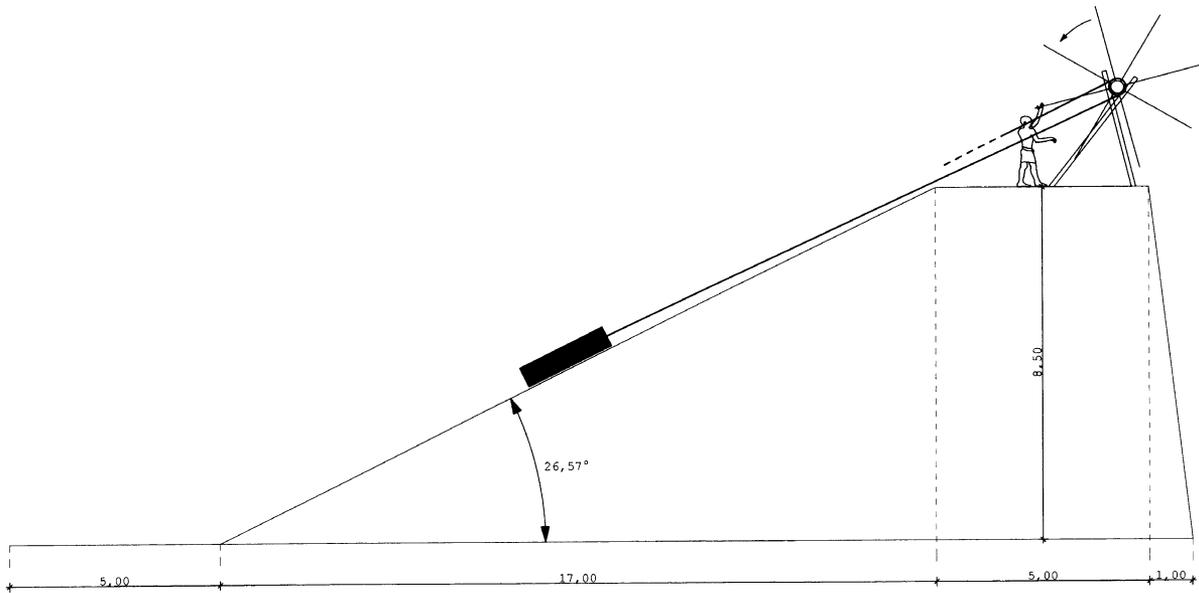
Fig. 12. Design of the winch at the top end of the ramp.
