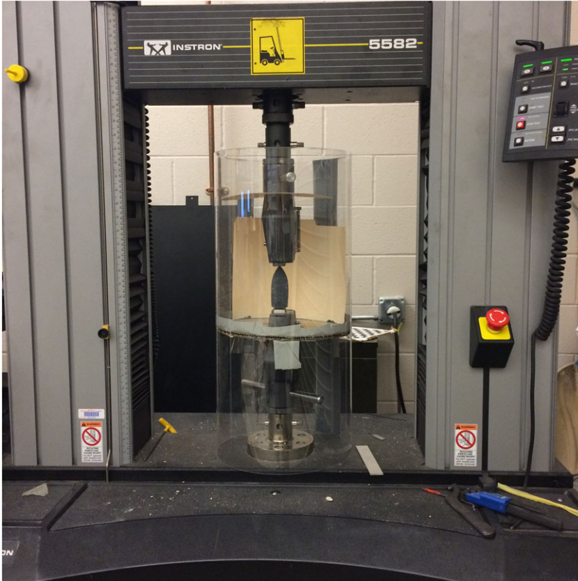
Figure 3 The static, compressive loading set-up using an Instron 5582 axial load frame. [Colour figure can be viewed at wileyonlinelibrary.com ]
