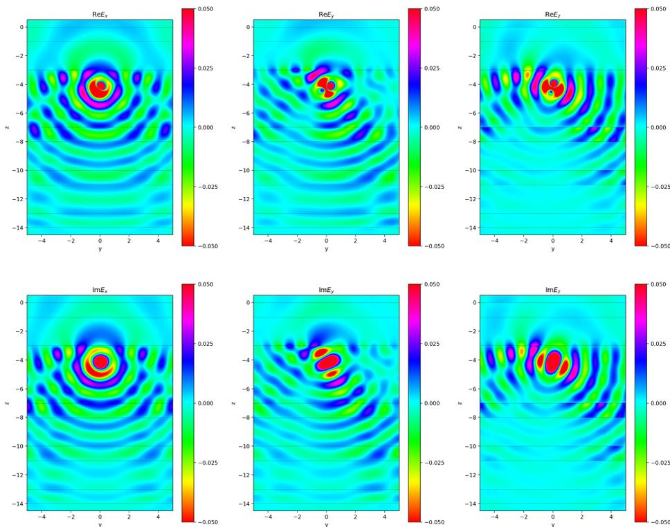
FIG. 4.1. Electric fields in a 10-layer medium described in section 4. Fields are computed along  $x = 0.2$  for  $-5.0 \leq y \leq 5.0$  and  $-14.5 \leq z \leq 0.5$ . The contouring level is clamped to the range  $(-0.05, 0.05)$  for a clearer illustration of wave pattern and avoiding the peak values near the source, which is located in the fourth layer at  $\mathbf{r}' = (0.0, 0.0, -4.23)$  with an orientation along the direction  $\hat{\alpha}' = (1/2, 1/2, 1/\sqrt{2})$ .
