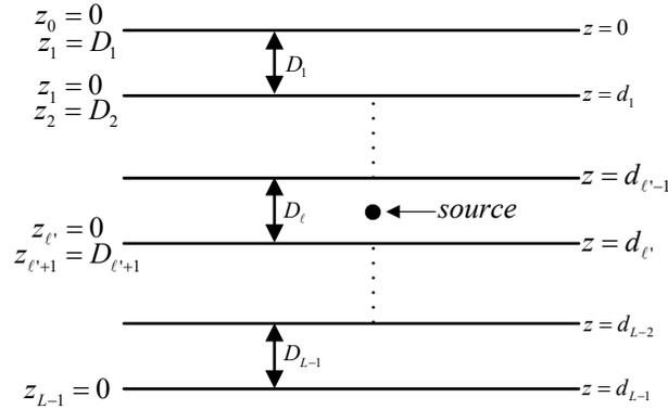
Figure 1: Sketch of the layer structure for general multi-layer media.
