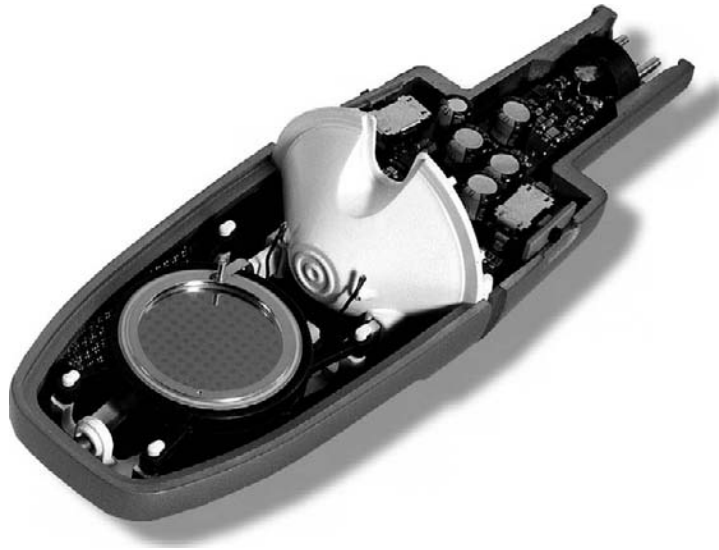
FIGURE 4.8 Inner detail of an AKG C3000B condenser mic. (Courtesy of AKG Acoustics, Inc., www.ake.com .)
