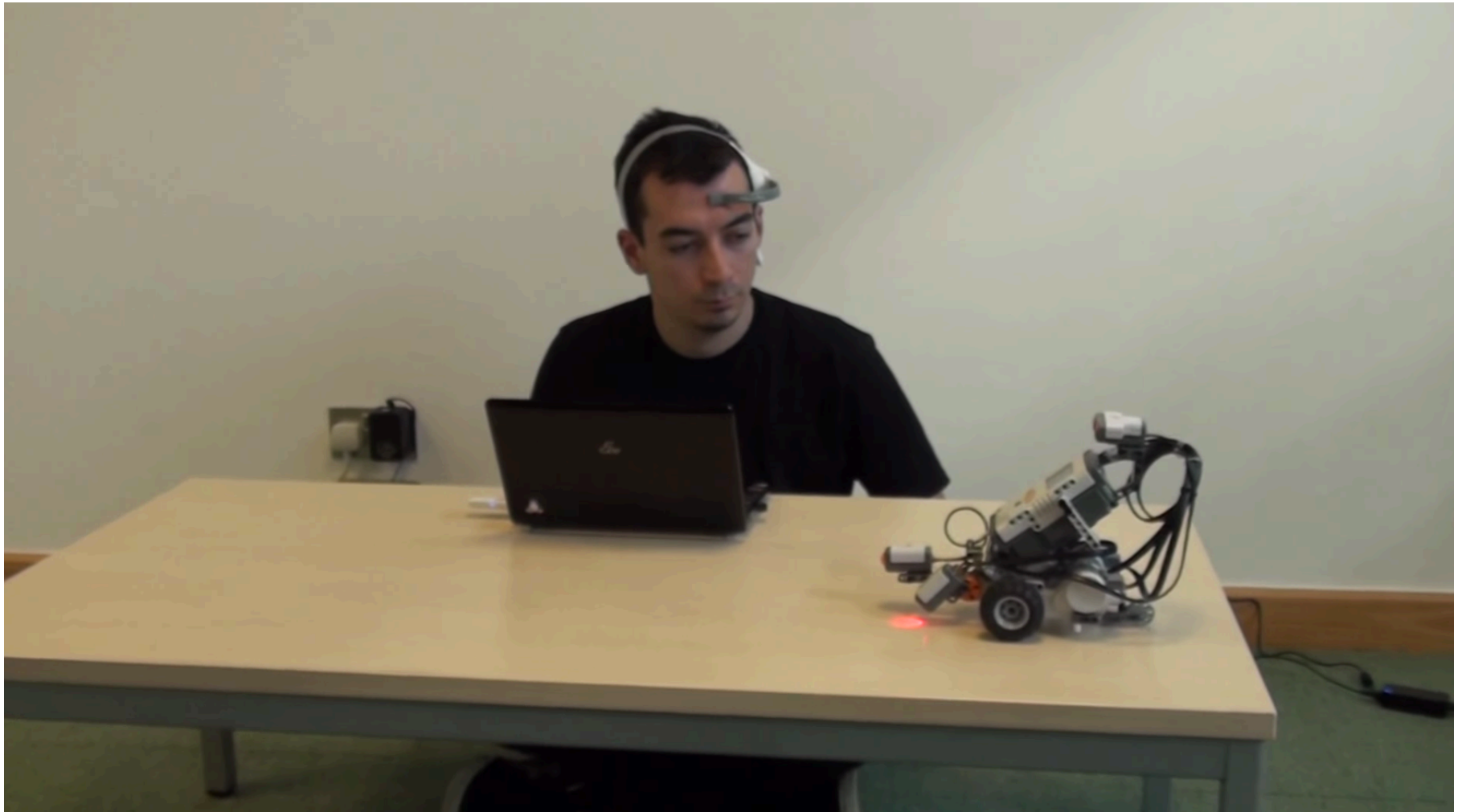
EEG sensor controlling the movement of a robot
