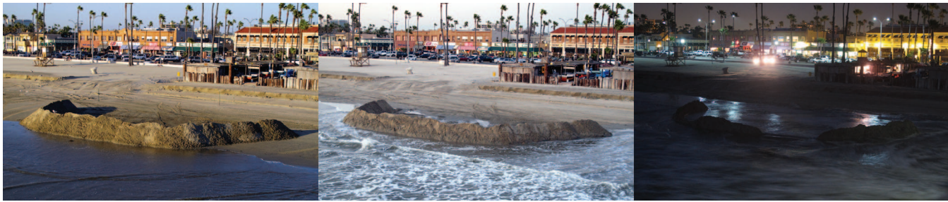
Figure 4. Photographs of berm 2 at (left to right) 1700, 1800, and 1830 show the progressive rise of the tide and erosion of the berm that occurred in each of the three experiments. (Color for this figure is available in the online version of this paper.)
