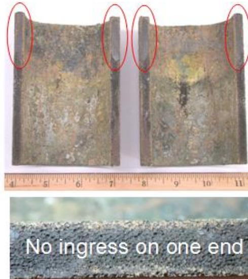
P/N 49A (4.5" long SiC foam infiltrated with **silica aerogel**) after 700°C PbLi exposure for 100 hours at 0.1 MPa
