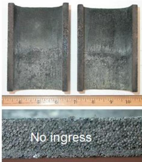
P/N 28A (4.5" long SiC foam infiltrated with **carbon aerogel**) after 700°C PbLi exposure for 100 hours at 0.1 MPa
