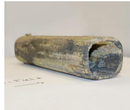
Picture of the FCI in the test section and after extracted from the duct.
