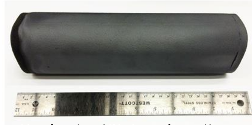
30 cm foam-based SiC FCI manufactured by Ultramed, USA
