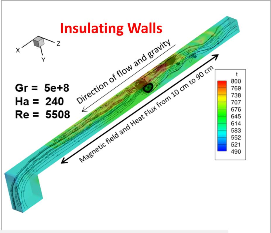
The velocity field shows **instabilities with flow reversals** that affect transport phenomena. These instabilities are **stronger for insulating walls** as compared to conducting walls due to lower Joule dissipation.
