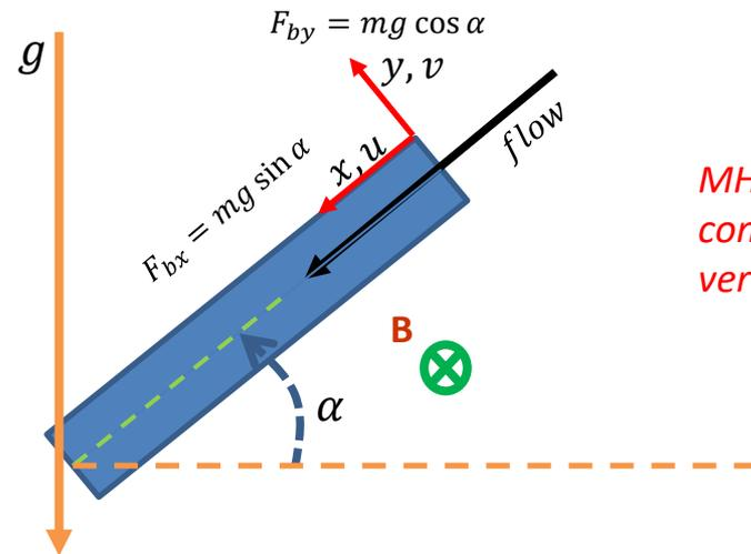
*Schematic illustrating the angle between the direction of gravity and fluid flow in the case of MHD convective flow in inclined ducts*
