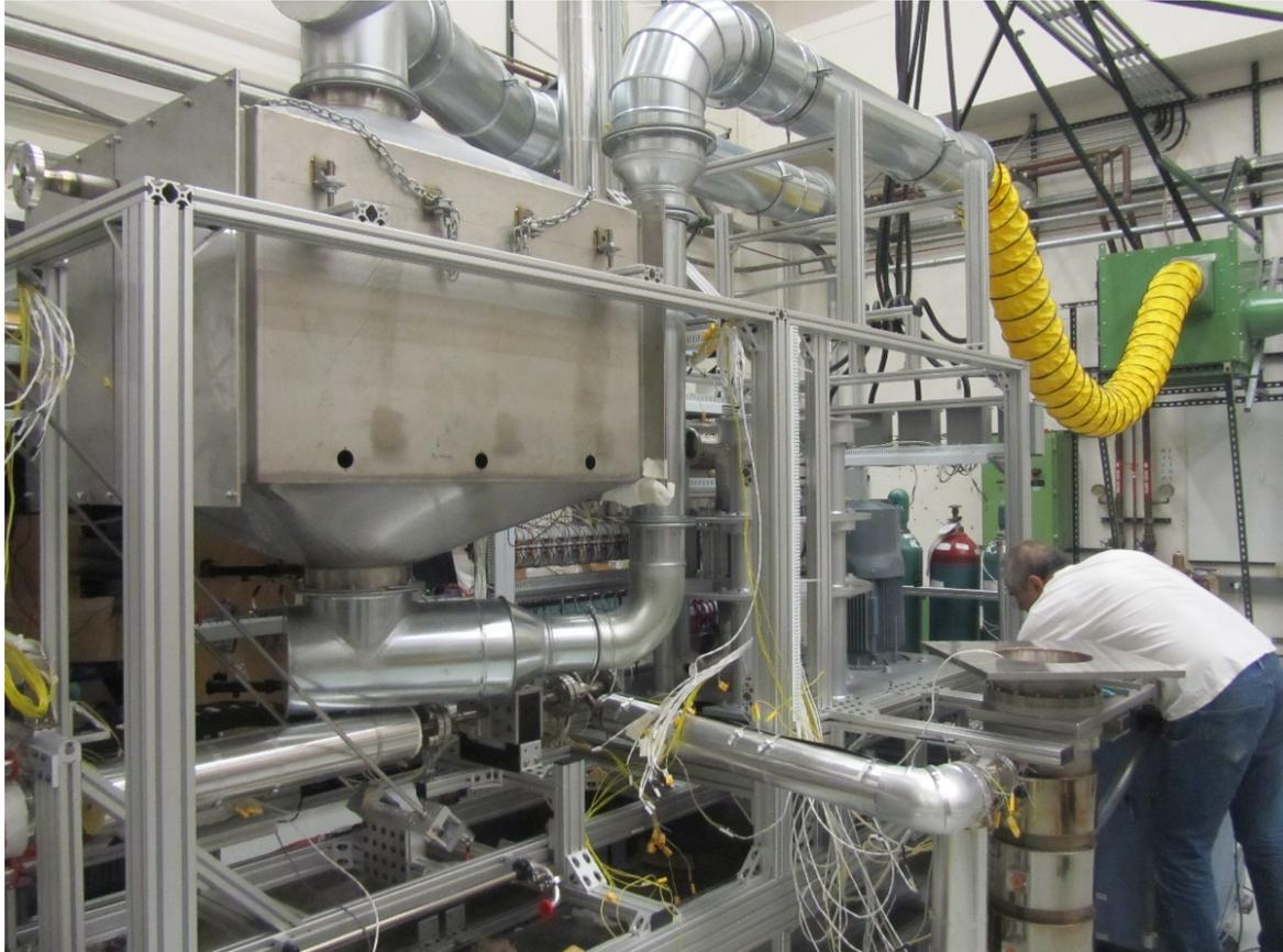
An air cooler was selected as heat rejection system for its simplicity and the capability to remove a large amount of power. In particular:
