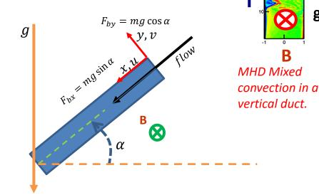
Schematic illustrating the angle between the direction of gravity and fluid flow in the case of MHD convective flow in inclined ducts
